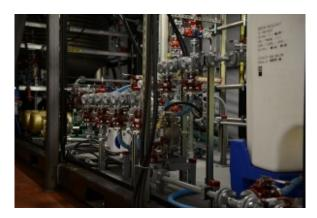
One of the two Field Deployable Hydrolysis Systems installed on the Cape Ray. I'll take the value of that over a crate of MANPADS any day. (US Army photo)
